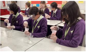
Polymers are molecules that are long chains, in this practical we use a borax solution and this forms links between the polymer chains in PVA
