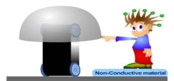
The way you may have seen static generated at school is with a **Van de Graaff Generator (see diagram).** The motor turns the rubber band and friction between the band and the rollers starts to build up huge amounts of charge.
