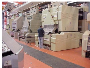
At the factory the gin sorts the seeds from the cotton.
