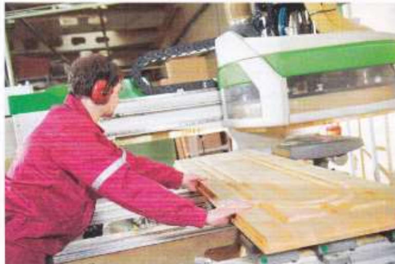
Industrial carpenter routing the detail into a wooden door
