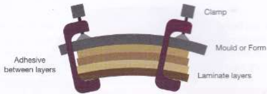
Material bent over a former and held in place with clamps
