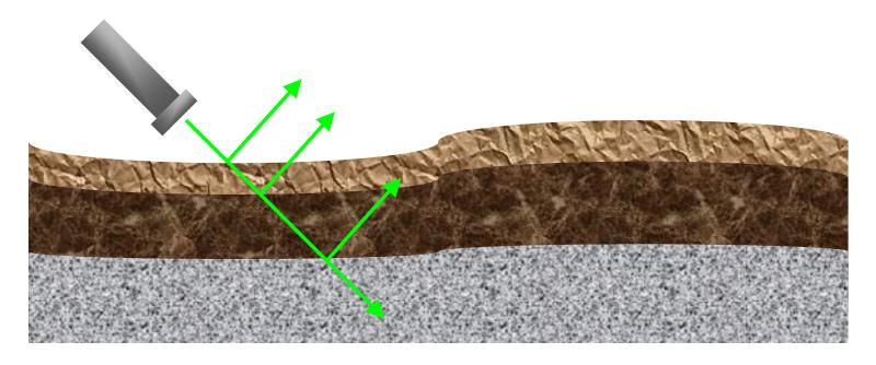
The device measures the time between sending the pulse and detecting its reflection. The speed of the ultrasound in the medium is known.
