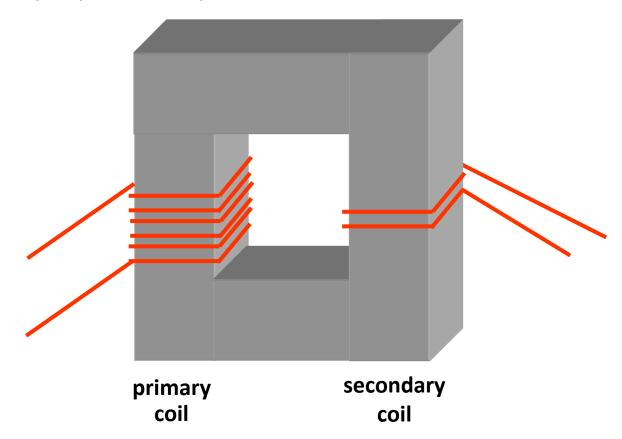
This a step-down transformer because there are less turns in the secondary coil than the primary coil.
