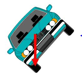
2. Centre of mass is directly above the edge of the wheelbase –car is on the point of toppling
