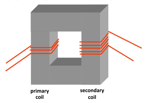
This a step-up transformer because there are more turns in the secondary coil than the primary coil.
