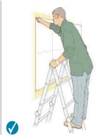
Correct – two clear rungs. Don't work any higher up this type of stepladder.
