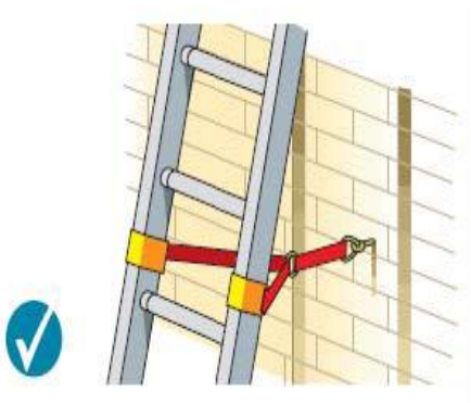
Tying near the base
