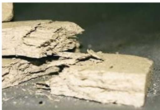
Pieces of Asbestos Insulating Board (AIB)
