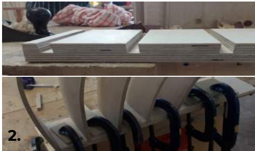
1. I firstly used PVA glue and lots of clamps to glue the base pieces together to create housing joints for the upright pieces.
