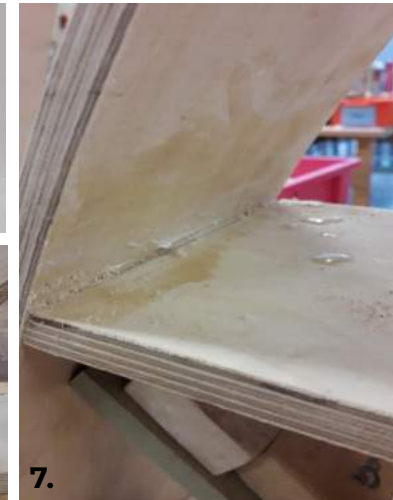
Then I cut the shelves and used the disc sander to create the angles so they fitted in between the upright pieces. I used PVA glue to attach them in place. Using a wet cloth and sand paper I cleaned up excess glue and sanded all surfaces to give a smooth finish.
