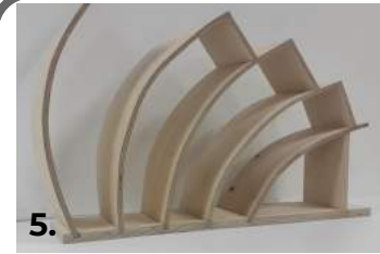
1. I firstly used PVA glue and lots of clamps to glue the base pieces together to create housing joints for the upright pieces.
