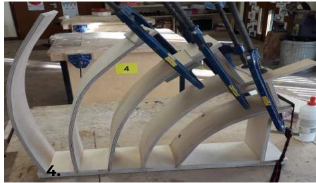
3. When the base was dry, I then cut the plywood pieces for the top with angled ends to fit tightly. I glued it all together with more PVA and clamps to hold it tight.
