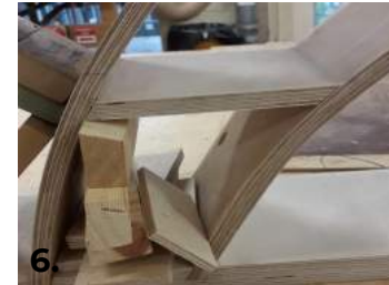
Then I cut the shelves and used the disc sander to create the angles so they fitted in between the upright pieces. I used PVA glue to attach them in place. Using a wet cloth and sand paper I cleaned up excess glue and sanded all surfaces to give a smooth finish.
