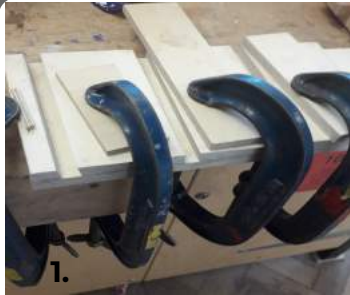
1. I firstly used PVA glue and lots of clamps to glue the base pieces together to create housing joints for the upright pieces.
