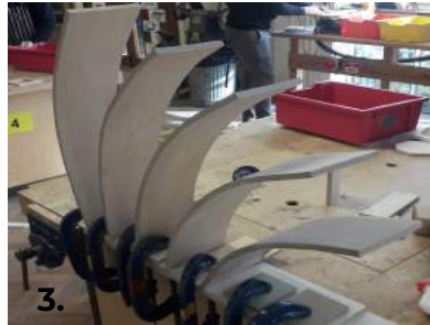
3. When the base was dry, I then cut the plywood pieces for the top with angled ends to fit tightly. I glued it all together with more PVA and clamps to hold it tight.
