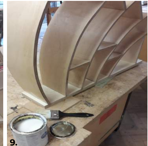
9. Finally, after sanding, I varnished the product to give it a better appearance that would also be more practical to clean rather than bare wood.
