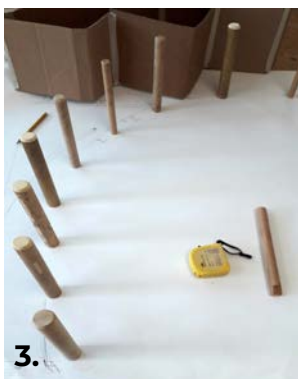
I firstly drew out my design, full scale, to get an idea for the exact curves I needed. Then I tried to make a universal curve which I could use to form all the curved pieces around, by glueing dowels in the shape of the curve. This curve is tighter at the top and shallower at the bottom so that all 5 different radii curves can be bent around it.
