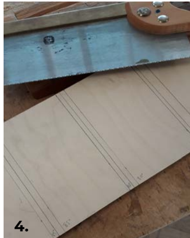
To make the base I used one solid length of 9mm plywood and another one cut at the correct angles and laminated on top create angled housing joints. I cut this piece up into sections and used the disc sander with an angled base to sand the angles into the pieces as shown above.
