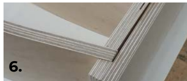
To make the base I used one solid length of 9mm plywood and another one cut at the correct angles and laminated on top create angled housing joints. I cut this piece up into sections and used the disc sander with an angled base to sand the angles into the pieces as shown above.
