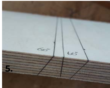
These pictures show how I worked out the angles to cut the ends of the plywood at from my scale drawing.
