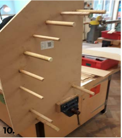
To securely attach the dowels I drilled holes in MDF to tightly fit them in. Above is a test piece to check for a tight fit. Also shown is a block that will attach to the back of the main piece of MDF to give a deeper hole to glue the dowel into.
